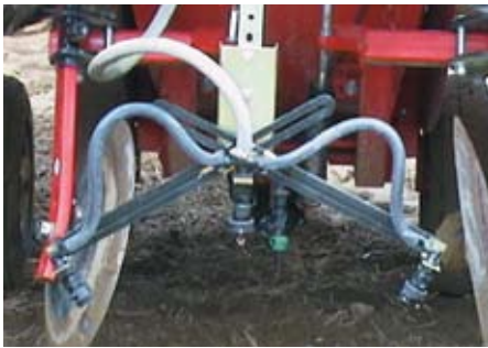
Overview of a three-nozzle herbicide banding system installed on a planter.
