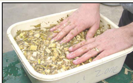
Figure 2. Gently agitating material to help the kernels sink to the bottom of the container.
