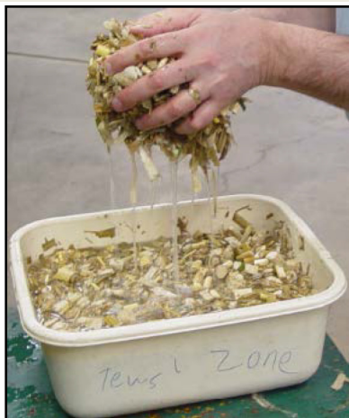
Figure 3. Skimming and removing the floating stover.
