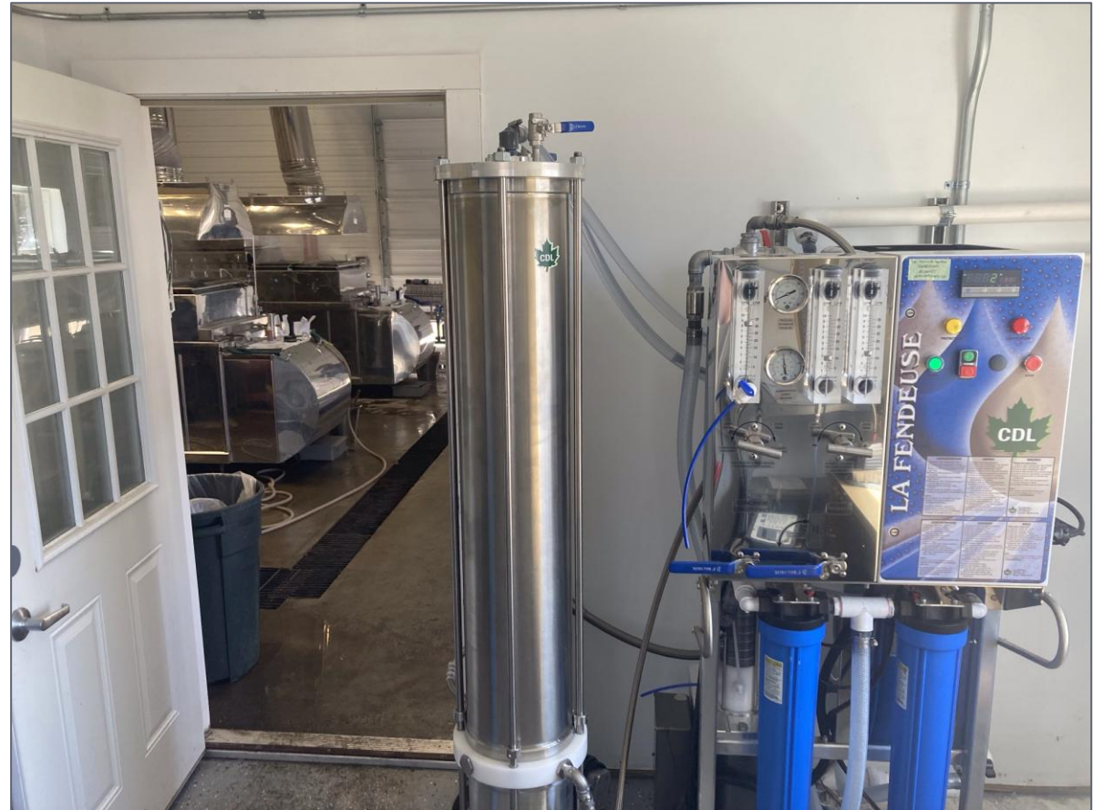
2 membranes, 1200 GPH, pompe de pression 7.5 HP
