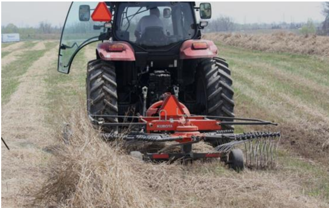
Figure 34. Switchgrass swath being raked in the spring. Tires, especially those on light farm equipment, can be vulnerable to puncture by the cut stems of switchgrass. Some farmers are filling their small implement tires with silicon to help prevent breakdowns from punctures.
