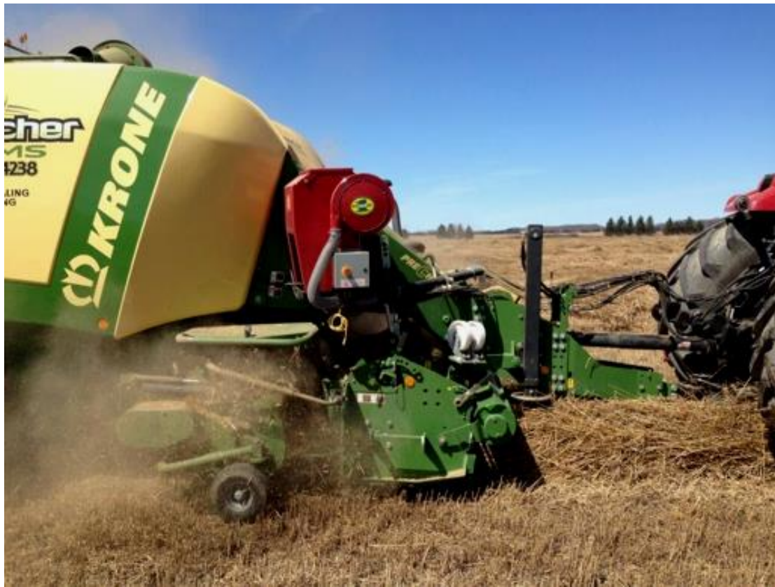
Figure 39. Close-up of Krone pre-chopper leaving fine particle dust in the field.
