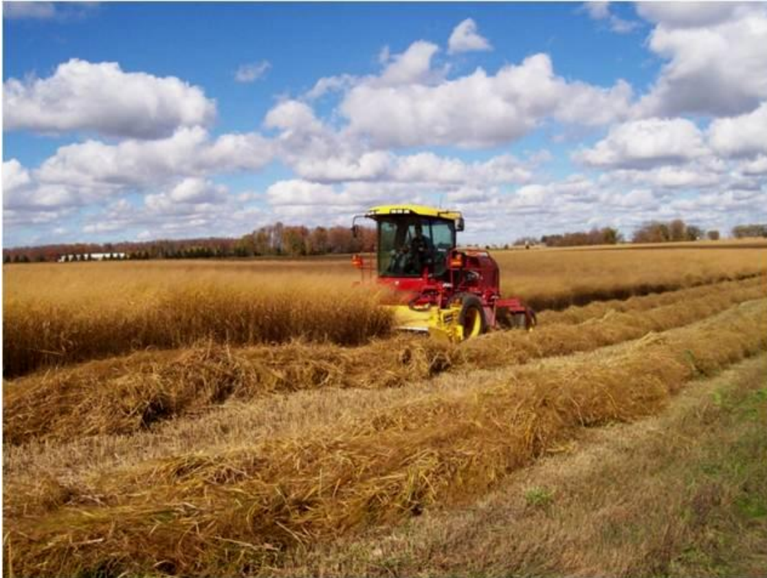
Figure 32. A self-propelled mower conditioner can be a good choice for heavy crops or for producers requiring a high throughput for larger acreages.
