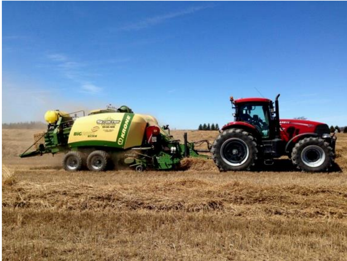
Figure 38. A large Krone baler with pre-chopper can process large volumes of switchgrass biomass in a day.
