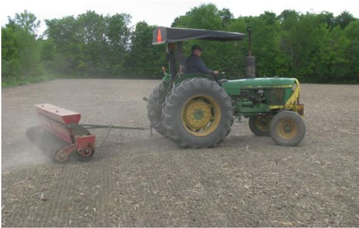
Figure 16. For most conventionally tilled soils, a Brillion seeder generally provides very good results for successful switchgrass establishment. It provides precise metering of the switchgrass seed, a uniform planting depth and a fine, firm seed bed for germination.
