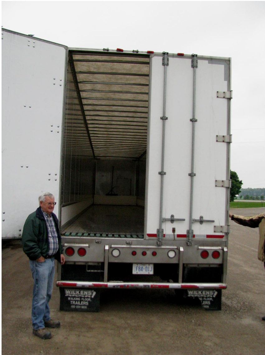
Figure 37. A transport truck with a walking floor can be a fast and safe means to load and unload bales. Many producers will make their square bales 7.5' long to enable transport in enclosed trailers.
