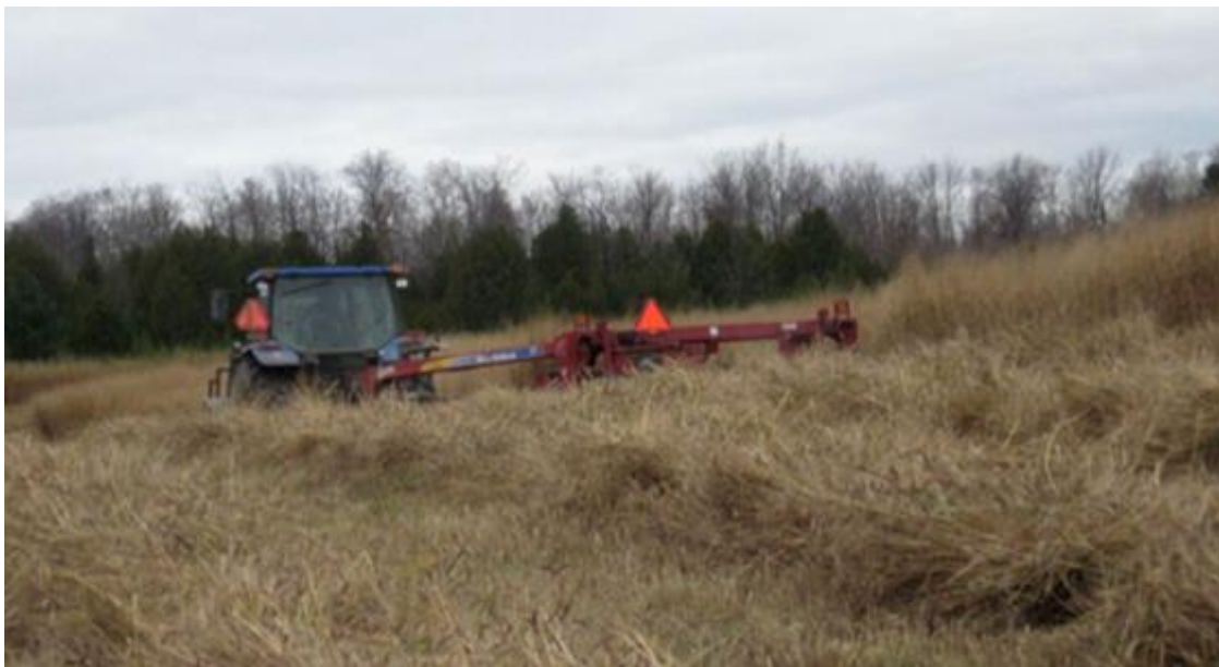
Figure 30. Mowing switchgrass in the fall with NH10' discbine. Growers should aim to achieve uniform, non-wavy windrows. The discbine speed of travel, cutting height, angle of the cutting bar and width of the swath all must be optimized. The goal should be to make as wide a swath as possible for the planned raking and baling operations. Avoid wavy windrows that have an uneven distribution of the biomass, as this will affect the drying speed and increase the chances of decay in the swath.
