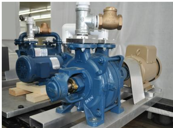
Figure 5.3 Pompe SiHi simple stage (-25 inHg)
