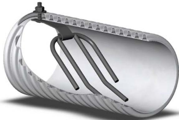
Figure 2 a: Removable grate with oscillating fork
